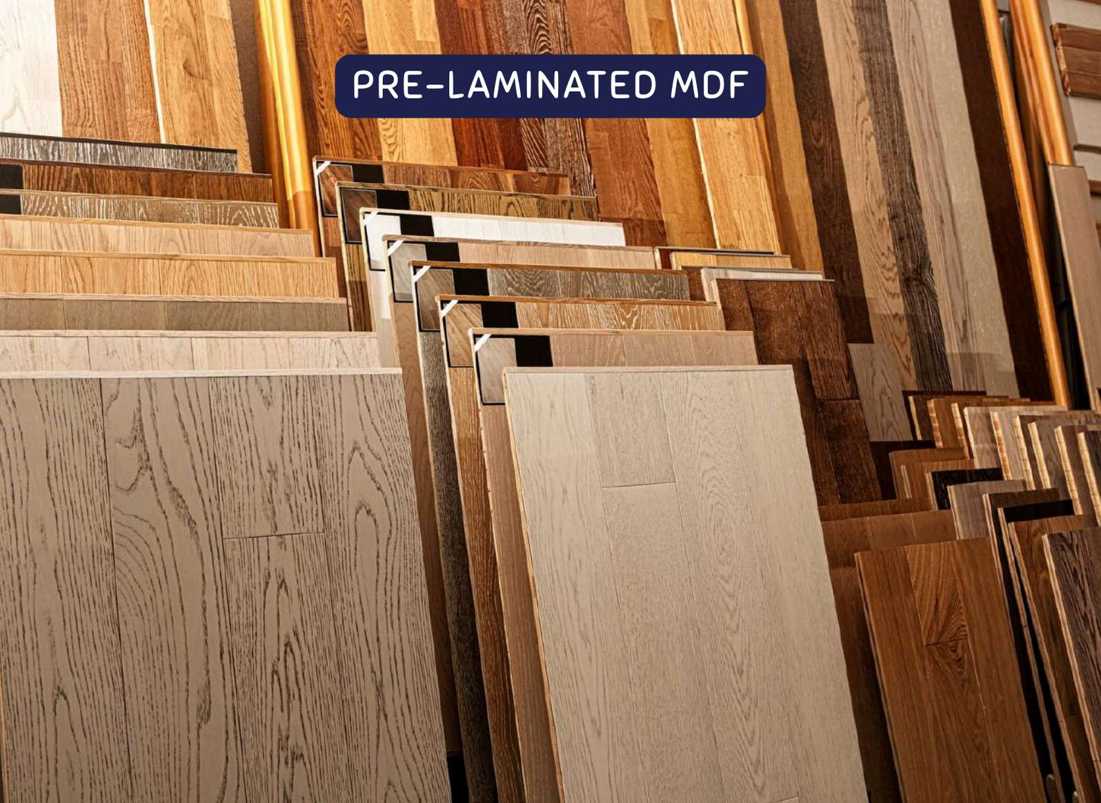
Pre-laminated MDF is Medium Density Fiberboard with decorative laminate or melamine film bonded on both sides, eliminating the need for additional finishing. It offers ready-to-use, smooth, and aesthetic panels for furniture and interiors.
